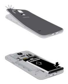
**Important**: Before closing the cover, check to see if there is any foreign substance such as dust or sand between the rubber on the back of the cover and the sealing area.
