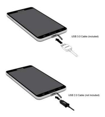
**Note:** Your phone supports USB 3.0 and USB 2.0, and includes a USB 3.0 cable for higher data transfer speeds when connected to another USB 3.0 device. You can also use USB 2.0 cables (not included) to charge and connect your phone.
