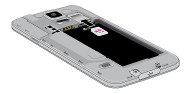
Carefully slide the SIM card into the SIM card slot.
